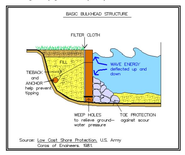
of bulkheads and seawalls can act to hasten erosion of beach areas immediately in front of the structures. This is because the structures redirect wave energy downward to the toe and beach areas. Bulkheads and seawalls are most appropriate where fishing and boating are the primary uses of the shore. They would not be appropriate on gently sloping beach areas.
