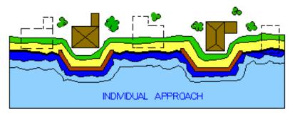
Individual approach to shoreline protection results in possible increased erosion risk to neighboring properties due to flanking of the bulkheads, a decrease in the number of desirable build—sites, and a disjointed, uneven shoreline.
